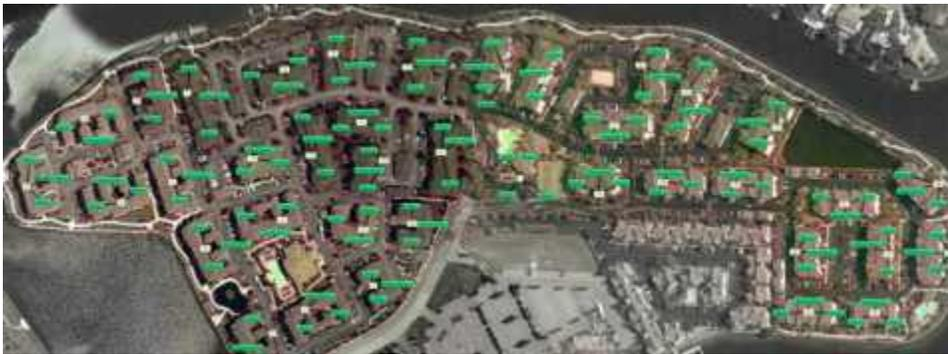
*O2 Connect's geographic network map displays subscribers in a residential area allowing technicians to note and fix performance issues before users are effected. Green color indicates that all is well. Yellow and orange would indicate poor or deteriorating performance. Red indicates an outage.*
