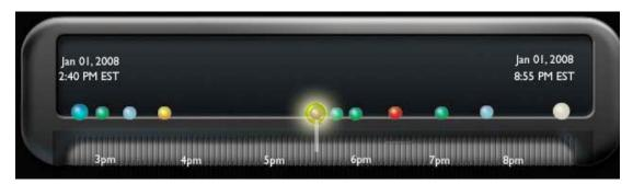
In this mockup the current production environment is represented by the white ball on the far right. The other balls represent ASEs that have been created over the previous six hours, with one ASE selected. ASEs are shown in different colors to represent their states, e.g. running, paused, etc.
